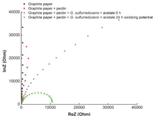
**Figure 5.** Nyquist graphs of graphite electrodes freshly coated with pectin and *G. sulfurreducens*, and the same electrodes after 24 h of incubation at +0.24 V versus SHE. While graphite paper in the absence of cells shows only diffusion-related resistance, the impedance of samples coated with living cells is typical of a charge transfer controlled process.
