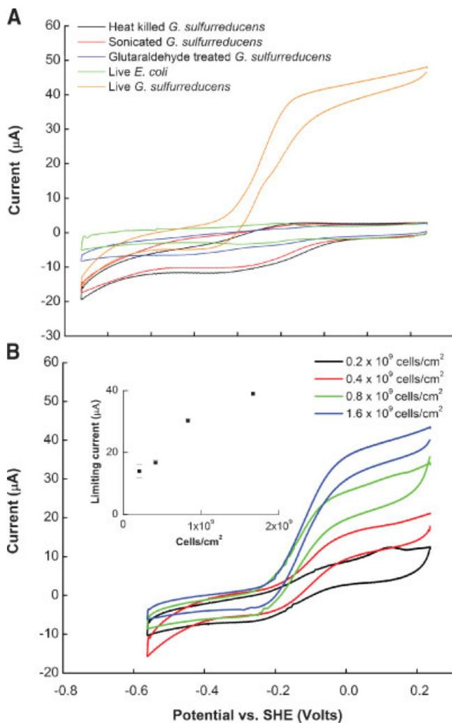
**Figure 2.** A: Current production by live versus killed *G. sulfurreducens* and *Escherichia coli* cells, as assayed by CV (10 mV/s), and (B) effect of increasing cell number at graphite electrodes (Inset: limiting current observed with increasing cell number, mean of three observations).
