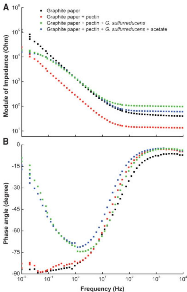
**Figure 4.** Bode graph (A) of graphite paper showing pure capacitive behavior of electrodes lacking cells, and changes in resistive behavior at low frequencies typical of charge transfer processes following addition of cells. Phase diagrams (B) for the same set of samples shows the effects of adding live cells at low frequencies ( $<10 \text{ Hz}$ ).
