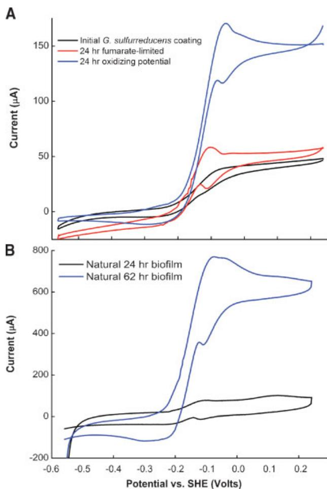
**Figure 3.** Typical current increase and change in CV features (10 mV/s) following incubation of electrodes containing (A) pectin-entrapped *G. sulfurreducens* for 24 h in the presence of acetate (10 mM) and limiting fumarate (2 mM) or under oxidizing conditions (at +0.24 V vs. SHE) (B) changes in voltammetry after growth of natural *G. sulfurreducens* biofilms on flat carbon electrode surfaces (+0.24 V vs. SHE) with no pectin entrapment.
