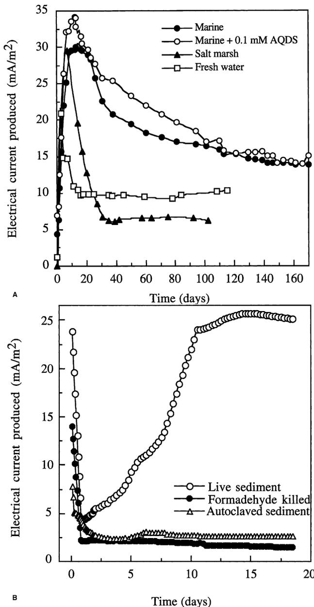
**Figure 1.** (A) Examples of current production by laboratory fuel cells constructed using sediments from three different sources under identical loads (1000 ohms), and effect of amending the marine sediments with 100  $\mu\text{M}$  AQDS. (B) Effect of sterilization on current production in laboratory marine sediment fuel cells.
