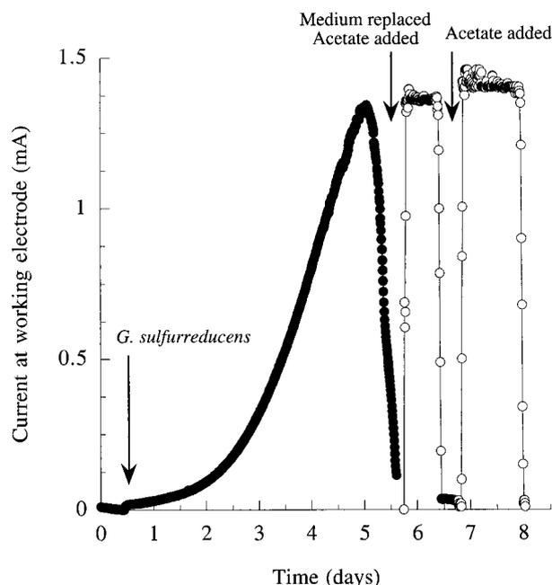
FIG. 4. Growth and current production by *G. sulfurreducens* in a chamber containing a graphite electrode poised at +200 mV versus an Ag/AgCl reference and effect of removing the growth medium and replacing it with anaerobic buffer plus acetate as the electron donor. Acetate (0.5 mM) was provided after replacing the medium, followed by a second pulse of 1 mM.
