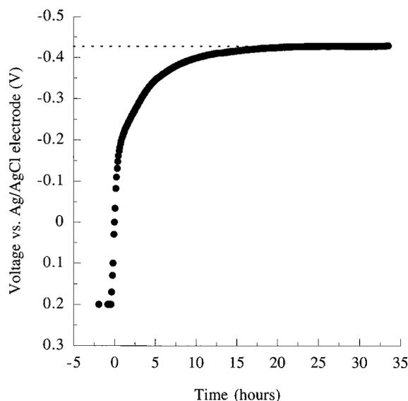
FIG. 7. Response of the graphite electrode potential to an attached population of *G. sulfurreducens* metabolizing acetate as the electron donor, after electrode control (poising by potentiostat) was switched off.
